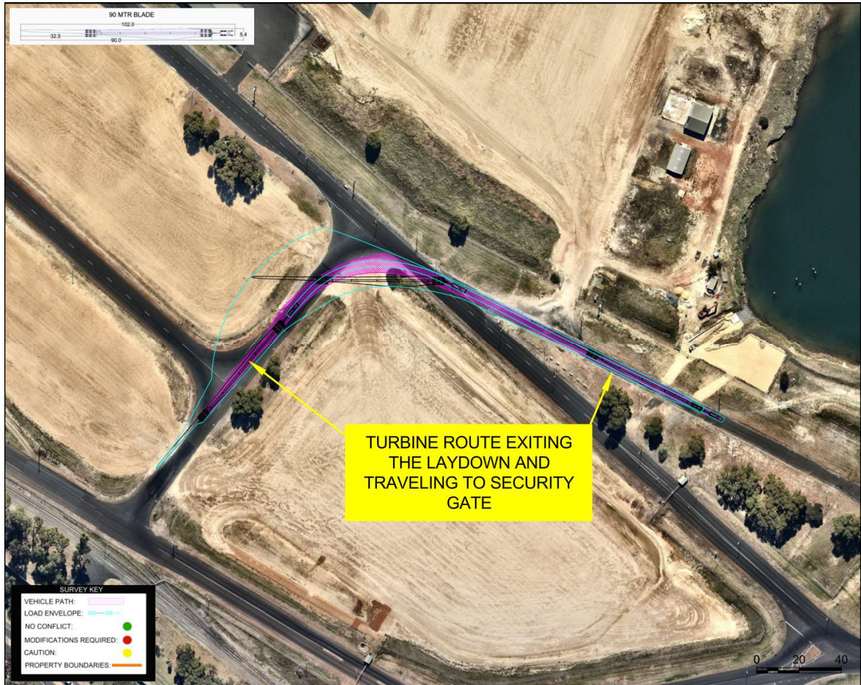
Figure 4 Laydown area through to security gate
