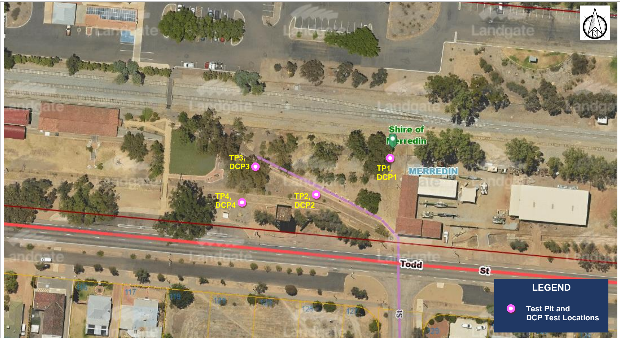
Site Sketch : Test Pits (TP) and Dynamic Cone Penetrometer (DCP) Test Locations
