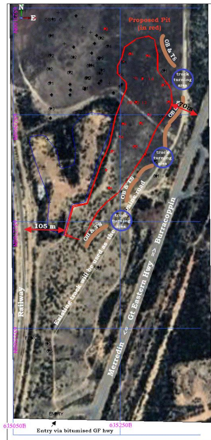
Figure 8 Burracoppin Gravel Pit - proximity to road & rail
